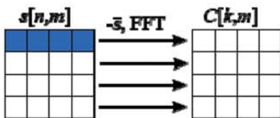
Fig. 3. Step 1: Fourier transform for all the Doppler frequency slices, where n is time, m – Doppler frequency, k – cadence frequency
