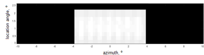
Figure 4. Radar portrait of an area with a shrub 3.9 m wide and 1.0 m high (model) at a distance of 10 m
