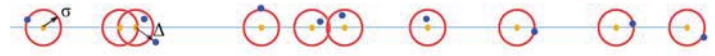
Figure 1. Subscribers' mutual placement type vector base model (reference line, blue) – a line or a group of lines describing the subscribers' coordinates mathematical expected value. The points describing the subscribers position have a random offset \Delta off the reference line. The red circles show the subscribers standard deviation \sigma off the reference line
