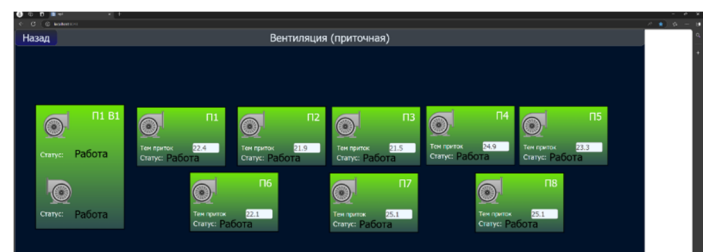
Fig. 8. General interface of the supply ventilation system
