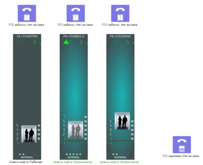
Fig. 17. Elevator equipment dispatching interface
