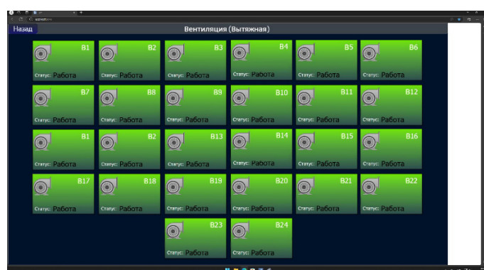
Fig. 10. General interface of the exhaust ventilation system
