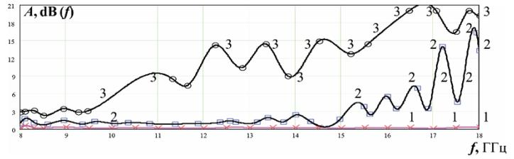
Fig. 11. Frequency response  $A$  (dB) when filling coaxial segment with oil ("2"), oil deposits ("3") and without filling ("1")
