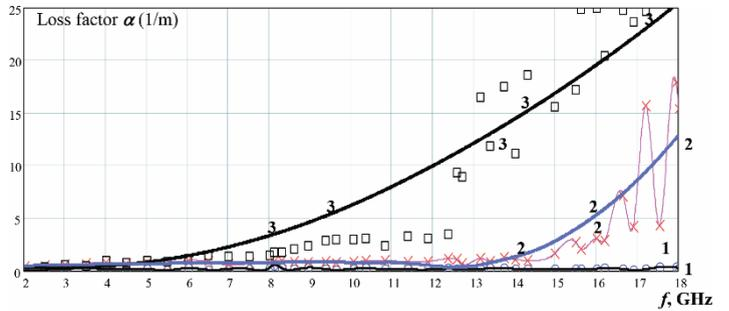
Fig. 12. Graph of the frequency dependence of the loss coefficient: 1 – in the clean segment, 2 – oil filling, 3 – when filling with oil deposits
