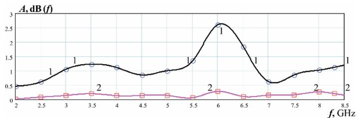
Fig. 6. Frequency response  $A$  (dB) when filled with oil (“1”) and without filling (“2”)
