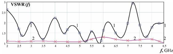
Fig. 7. VSWR ( $f$ ) when filling the segment with oil deposits ("1") and without filling ("2")
