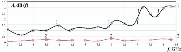
Fig. 8. Frequency response  $A$  (dB) when filling the segment with oil deposits ("1") and without filling ("2")
