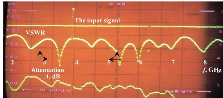
Fig. 4. Photo of the meter screen (P2-103) for the coaxial segment filled with oil deposits
