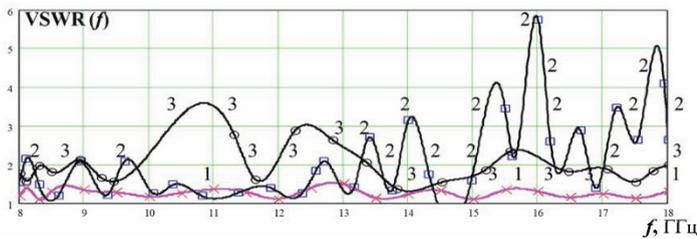
Fig. 10. VSWR ( $f$ ) dependence when filling coaxial segment with oil ("2"), oil deposits ("3") and without filling ("1")
