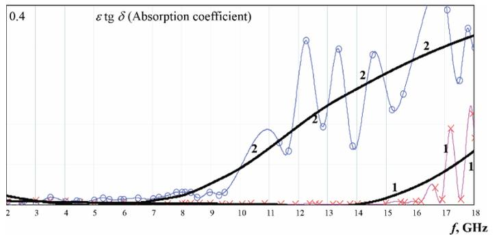
Fig. 13. Graph of the frequency dependence of the absorption coefficient: 1 – for oil filling, 2 – for filling with oil deposits
