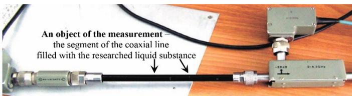
Fig. 2. The object of the measurement
