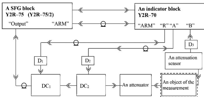
Fig. 3. A scheme of the experimental set with VSWR measuring instrument R2-103 (R2-104)
