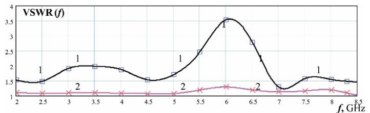
Fig. 5. VSWR ( $f$ ) when filled with oil (“1”) and without filling (“2”)
