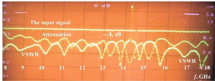
Fig. 9. Photo of the meter screen (P2-104) for a coaxial segment filled with oil deposits
