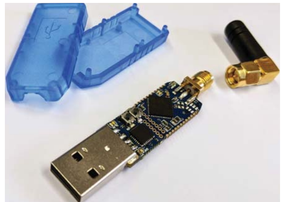
Fig. 2. CC2652R microcontroller development board with an aerial
