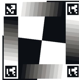
Fig. 3. High contrast Slanted edge pattern with ArUco alignment markers and OECF estimation regions
